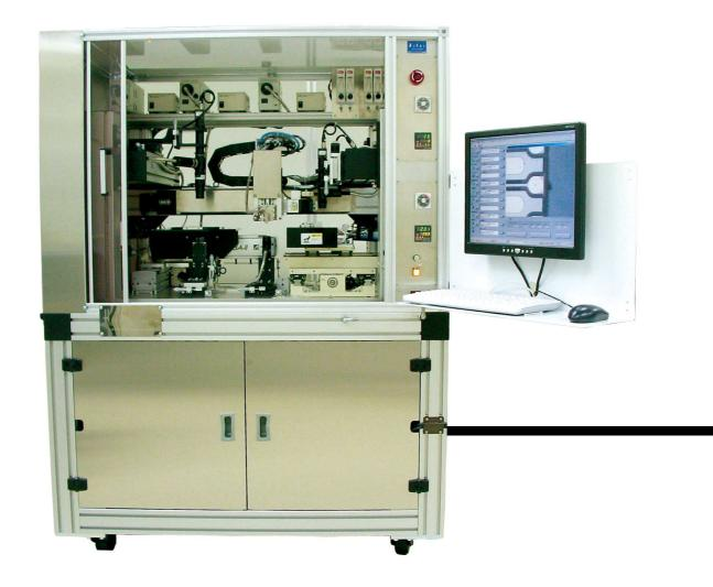
Most suitable for small lot product packaging and can be used for all methods such as bond, eutectic, ultrasonic, and thermocompression.
